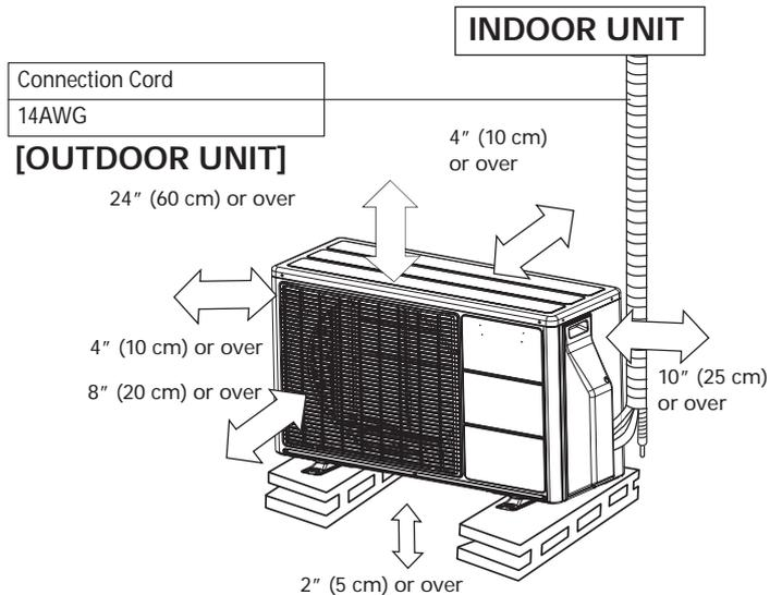
• Do not directly install it on the ground, otherwise it will cause failure.
