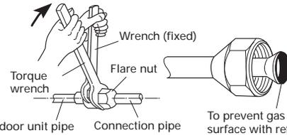
To prevent gas leakage, coat the flare surface with refrigerant oil.
