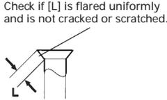
Insert the flare nut (always use the flare nut attached to the indoor and outdoor units respectively) onto the pipe and perform the flare processing with a flare tool.
